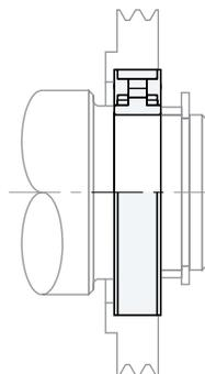
The ASK clutch must be mounted with a press fit on both the outer and inner race. The shaft diameter tolerance must be held to h6 or j6. The bore of the housing for the outer race should be a K6 tolerance.
