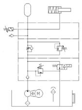
Fig 3. Fast Approach Soft Braking
