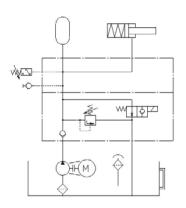
Top module: Test point, pressure switch and accumulator.
