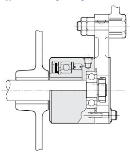
The Model FS clutches require a snap-ring bearing (furnished by customer) mounted in the open end of the clutch as shown. An adequate seal or cover must be provided at the open end to retain lubricant. The shaft end must be turned down or threaded to accommodate the bearing or lock nut. All fasteners are recommended to be grade 8 bolts.
