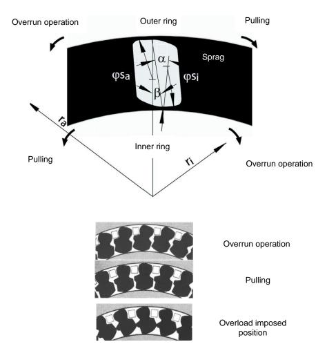
Fig. 2 Pulling/overrun operation
