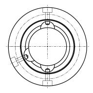
Fig. 3 Position of oil filling plugs
