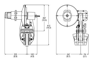
Maximum Braking Force = 6kN (1348.85 lbf) Weight of caliper and actuator - 17.9kg (39.46 lb)
