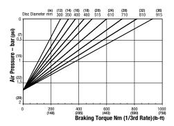
Minimum Pressure for full retraction: 1.7 bar (25 psi) Maximum Braking Force 1/3 rate: 2.2kN (497.57 lbf) Weight of caliper and thruster - 10.5kg (28.14 lb)
