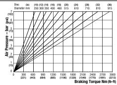
Maximum Pressure 7 bar (102 psi) Maximum Braking Force = 6.9kN @ 7 bar (1551.18 lbf @ 102 nsi) Weight of MR caliper and thruster - 7.82kg (17.24 lb)
