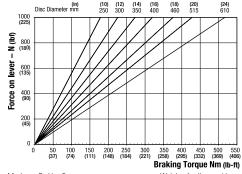
Maximum Braking Force = 1.88kN @ 0.8kN force on lever (422.64 @ 179.84 lbf) Weight of caliper and lever assembly - 2.13kg (4.69 lb) Weight of lever assembly only - 0.63kg (1.39 lb)
