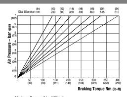
Maximum Braking Force = 1.44kN @ 7 bar (323.72 @ 102 psi) Weight of caliper and thruster – 2.5kg (5.51 lb)
