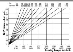
Maximum Pressure 7 bar (102 psi) Maximum Braking Force = 3.5kN @ 7 bar (786.83 @ 102 psi) Weight of MR caliper and thruster - 7.65kg (16.87lb)
