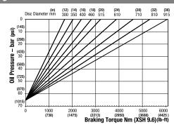
Minimum Pressure for full retraction: 82 bar (1189 psi) Maximum Braking Force XSH 9.6: 14.3kN (3214.76 lbf) Weight of caliper and thruster - 11.6kg (25.57 lb)
