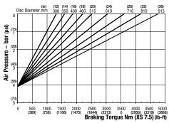
Minimum Pressure for full retraction: 5.5 bar (80 psi) Maximum Braking Force XS 7.5: 11.2kN (517.86 lbf) Weight of caliper and thruster - 11.9kg (26.23 lb)
