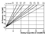
Maximum Braking Force S 12.9: 30kN (6744.27 lbf) Minimum Pressure for full retraction: 7 bar (102 psi) Weight of caliper and thruster - 48kg (105.82 lb) Weight of thruster only - 14kg (30.86 lb) Volume displacement of thruster at full retraction = 1.31ml (0.04 fl oz)
