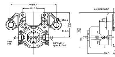
The Twiflex VCS-FL disc brake caliper comprises a single spring module forming the 'active' side of this floating unit and is available for use where space is limited or to accommodate axial disc float of ±6mm (0.24 in).
