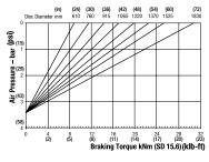
Maximum Braking Force SD 15.6: 36kN (8093.12 lbf) Minimum Pressure for full retraction: 4.6 bar (67 psi) Weight of caliper and thruster - 55kg (121.25 lb) Weight of thruster only - 21kg (46.29 lb) Volume displacement of thruster at full retraction = 2.5fml (0.08 fl oz)
