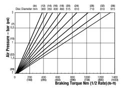
Minimum Pressure for full retraction: 2.5 bar (36 psi) Maximum Braking Force 1/2 rate: 3.2kN (719.38 lbf) Weight of caliper and thruster - 10.5kg (23.14 lb)
