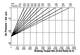
Minimum Pressure for full retraction: 3.3 bar (48 psi) Maximum Braking Force 2/3rd rate: 4.3kN (996.67 lbf) Weight of MR caliper and thruster - 10.0kg (22.04 lb) Weight of MR2 caliper and thruster - 10.5kg (23.14 lb) Weight of thruster only - 3.5kg (7.71 lb) Volume displacement of thruster at full retraction is 950ml (32.12 lb)
