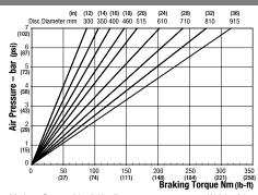
Maximum Pressure 7 bar (102 psi) Maximum Braking Force = 0.74kN @ 7 bar (? @ 102 psi) Weight of caliper and thruster - 7.34kg (16.18 lb) Weight of thruster only - 0.34kg (0.74 lb) Volume displacement of thruster at full stroke = 25ml (0.84 fl oz)
