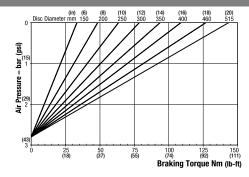
Maximum Pressure = 7 bar (102 psi) Minimum Pressure for full retraction = 4.3 bar (62.37 psi) Maximum Braking Force = 0.6kN (134.89 lbf) Weight of caliper and thruster – 1.36kg (3.00 lb) Weight of thruster only – 0.61kg (1.34 lb) Volume displacement of thruster at full retraction = 20ml (0.68 fl oz)
