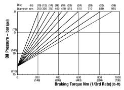
Minimum Pressure for full retraction: 17 bar (247 psi)
