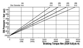
Maximum Braking Force XSH 9.6: 14.3kN (3214.77 lbf) Minimum Pressure for full retraction: 82 bar (1189 psi) Weight of caliper and thruster - 13.82kg (30.47 lb)
