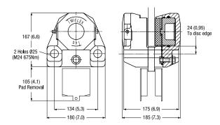
The Twiflex T40 disc brake caliper is split caliper design suitable for use with a minimum disc thickness of 20mm (0.79 in). The modules are mounted each side of a central mounting plate of the same thickness as the brake disc. Minimum disc diameter is 300mm (11.81 in).
