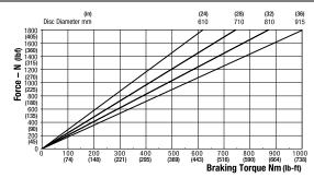
Weight of caliper and hand wheel assembly - 10.52kg (23.19 lb) Weight of hand wheel assembly only - 1.3kg (2.87lb) Maximum Braking Force = 2.68kN (602.49 lbf)
