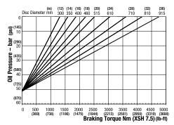
Minimum Pressure for full retraction: 65 bar (943 psi) Maximum Braking Force XSH 7.5: 11.2kN (2517.86 lbf) Weight of caliper and thruster - 11.4kg (25.13 lb)
