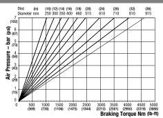
Maximum Pressure 7 bar (102 psi) Maximum Braking Force = 10.8kN @ 7 bar (2427.97 lbf @ 102 psi) Weight of MR caliper and thruster - 8.56kg (18.87 lb) Weight of MR2 caliper and thruster - 9.06kg (19.97 lb) Weight of thruster only - 2.06kg (4.54 lb) Volume displacement of thruster at full stroke = 426ml (14.40 fl oz)
