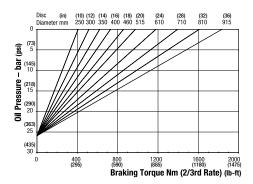
Minimum Pressure for full retraction 33 bar (429 psi) Maximum Braking Force 2/3rd rate: 4.3kN (996.67 lbf) Weight of MR caliper and thruster - 10.5kg (23.14 lb) Weight of MR2 caliper and thruster - 11kg (24.25 lb) Weight of thruster only - 4kg (8.81 lb) Volume displacement of thruster at 4mm (0.16 in) retraction = 5ml (0.16 oz)
