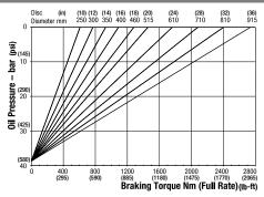
Minimum Pressure for full retraction: 50 bar (725 psi) Maximum Braking Force full rate: 6.4kN (1438.17 lbf) Weight of MR caliper and thruster - 10.5kg (23.14 lb) Weight of MR2 caliper and thruster - 11kg (24.25 lb)
