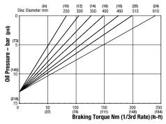
Maximum Braking Force 1/3rd rate: 0.87kN (195.58 lbf) Minimum Pressure for full retraction: 17 bar (247 psi) Weight of caliper and thruster - 5.5kg (12.13 lb) Weight of thruster only - 4kg (8.82 lb) Volume displacement of thruster at 4mm (0.16 in) retraction = 5ml (0.17 fl oz)
