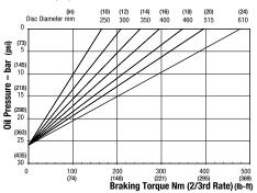
Maximum Braking Force 2/3rd rate: 1.74kN (391.17lbf) Minimum Pressure for full retraction: 33 bar (479 psi) Weight of caliper and thruster - 5.5kg (12.13 lb) Weight of thruster only - 4kg (8.82 lb) Volume displacement of thruster at 4mm (0.16 in) retraction = 5ml (0.17 fl oz)
