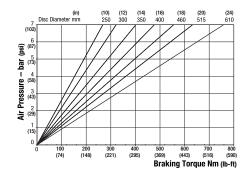
Maximum Pressure 7 har (102 psi) Maximum Braking Force = 2.76kN @ 7 bar (620.47 lbf @ 102 psi)
