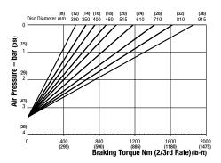
Minimum Pressure for full retraction: 3.3 bar (48 psi) Maximum Braking Force 2/3 rate: 4.3kN (966.67 lbf) Weight of caliper and thruster - 10.5kg (23.14 lb)
