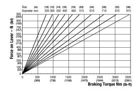
Weight of MR caliper and thruster - 7.9kg (17.41 lb) Weight of MR2 caliper and thruster - 8.4kg (18.51 lb) Weight of lever assembly only - 1.4kg (3.08 lb) Maximum Braking Force = 8.3kN @ 0.9kN 1865.91 @ 202.33 lbf) force on lever
