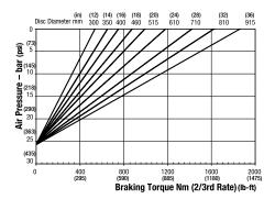
Minimum Pressure for full retraction: 33 bar (479 psi) Maximum Braking Force 2/3 rate: 4.3kN (966.67 lbf) Weight of caliper and thruster - 11kg (24.25 lb) Weight of thruster only - 4.0kg (8.81 lb) Volume displacement of thruster at 4mm (0.16 in) retraction = 5ml (0.16 fl oz)
