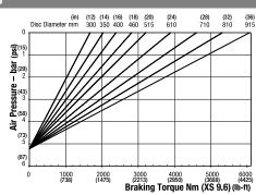
Minimum Pressure for full retraction: 6.4 bar (93 psi) Maximum Braking Force XS 9.6: 14.3kN (3214.76 lbf) Weight of caliper and thruster - 12.1kg (26.67 lb)
