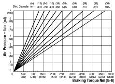
Maximum Pressure 7 bar (102 psi) Maximum Braking Force = 11kN @ 7 bar (2472.89 @ 102 psi) Weight of caliper and thruster - 9.06kg (19.97 lb)
