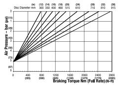
Minimum Pressure for full retraction: 5 bar (73 psi) Maximum Braking Force full rate: 6.4kN (1438.77 lbf) Weight of caliper and thruster - 10.5kg (23.14 lb)
