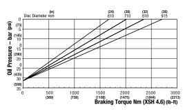
Maximum Braking Force XSH 4.6: 6.8kN (1528.70 lbf) Minimum Pressure for full retraction: 40 bar (580 psi) Weight of caliper and thruster - 13.22kg (29.15 lb)
