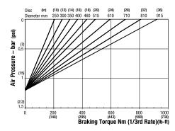
Minimum Pressure for full retraction: 1.7 bar (25 psi) Maximum Braking Force 1/3rd rate: 2.2kN (494.57 lbf) Weight of MR caliper and thruster - 10.0kg (22.04 lb) Weight of MR2 caliper and thruster - 10.5kg (23.14 lb) Weight of thruster only - 3.5kg (7.71 lb) Volume displacement of thruster at full retraction is 950ml (32.12 fl oz)
