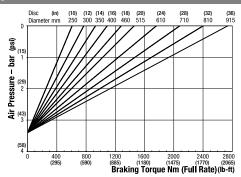
Minimum Pressure for full retraction: 5 bar (73 psi) Maximum Braking Force full rate: 6.4kN (1438.77 lbf) Weight of MR caliper and thruster - 10.0kg (22.04 lb) Weight of MR2 caliper and thruster - 10.5kg (23.14 lb) Weight of thruster only - 3.5kg (7.71 lb) Volume displacement of thruster at full retraction is 950ml (32.12 fl oz)
