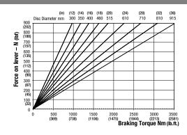
Weight of caliper and lever assembly - 8.4kg (18.51 lb) Weight of lever assembly only - 1.4kg (3.08 lb) Maximum Braking Force = 8.3kN @ 0.9kN force on lever (1865.91 @ 202.32 lbf force on lever)
