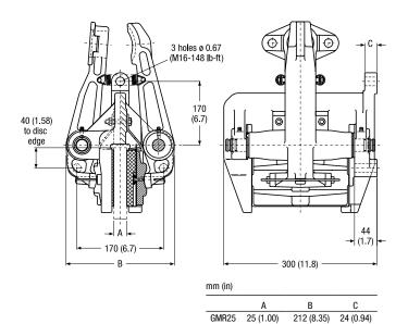
The Twiflex GMR and GMR40 series of disc brake calipers are suitable for use with discs of 25.4mm (1 in), and 40mm (1.57 in)thick respectively. Minimum disc diameter is 610mm (24.02 in).
