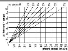
Maximum Pressure 7 bar (102 psi) Maximum Braking Force = 0.76kN @ 7 bar (170.85 lbf @102 psi) Weight of caliper and thruster - 1.89kg (4.17 lb) Weight of thruster only - 0.39kg (0.86 lb) Volume displacement of thruster at full stroke = 21ml (0.71 fl oz)
