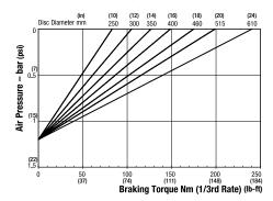
Maximum Braking Force 1/3rd rate: 0.87kN (195.58 lbf) Minimum Pressure for full retraction: 1.7 bar (25 psi) Weight of caliper and thruster - 4.9kg (10.80 lb) Weight of thruster only - 3.4kg (7.49 lb) Volume displacement of thruster at full retraction = 950ml (32.12 fl oz)
