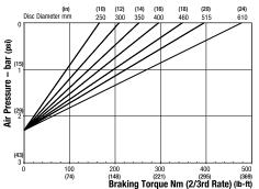
Maximum Braking Force 2/3rd rate: 1.74kN (391.17 lbf) Minimum Pressure for full retraction: 3.3 bar (48 psi) Weight of caliper and thruster - 4.9kg (10.80 lb) Weight of thruster only - 3.4kg (7.49 lb) Volume displacement of thruster at full retraction = 950ml (32.12 fl oz)
