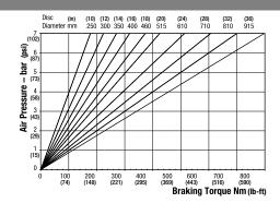
Maximum Pressure 7 bar (102 psi) Maximum Braking Force = 1.9kN @ 7 bar (427.14 lbf @ 102 psi) Weight of MR caliper and thruster - 6.8kg (14.99 lb) Weight of MR2 caliper and thruster - 7.3kg (16.09 lb) Weight of thruster only - 0.3kg (0.66 lb) Volume displacement of thruster at full stroke = 64ml (2.16 fl oz)
