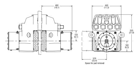
The Twiflex VMS3-SPS disc brake caliper is comprised of two modules bolted to a central mounting plate, 12mm (0.47 in) thicker than the brake disc. Minimum disc thickness is 38mm (1.49 in) and minimum disc diameter is 1500mm (59.06 in) with no maximum except for practical limitations. Based on a development of the earlier Twiflex VMS2-SP disc brake, the VMS3-SPS provides a significant increase in braking force but in a similarly sized package.
