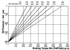
Maximum Braking Force full rate: 2.6kN (584.50 lbf) Minimum Pressure for full retraction: 50 bar (725 psi) Weight of caliper and thruster - 5.5kg (12.13 lb) Weight of thruster only - 4kg (8.82 lb) Volume displacement of thruster at 4mm (0.16 in) retraction = 5ml (0.17 fl oz)
