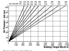
Maximum Pressure 7 bar (102 psi) Maximum Braking Force = 3.6kN @ 7 bar (809.31 lb @ 102 psi) Weight of caliper and thruster - 8.15kg (17.96 lb)
