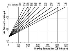
Minimum Pressure for full retraction: 3.1 bar (45 psi) Maximum Braking Force XS 4.6: 6.8kN (528.70 lbf) Weight of caliper and thruster - 11.5kg (25.35 lb)
