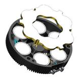
Lift the two piston assemblies (11) highlighted in the below image to allow removal of the pneumatic tubes from the barbed connectors attached to the cover (15), once these tubes are free all of the piston assemblies can be lifted out along with the connected tubes and fittings.
