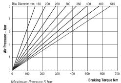
Maximum Braking Force = 2.75kN@ 5 bar Weight of caliper and thruster - 1.9kg
