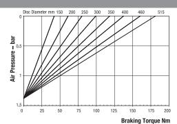
Maximum Pressure = 7 bar Minimum Pressure for full retraction = 1.75 bar Maximum Braking Force = 0.76kN Weight of caliper and thruster – 2.2kg Weight of thruster only – 1.45kg Volume displacement of thruster at full retraction = 46ml
