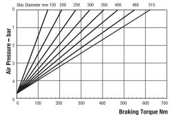
Maximum Pressure = 7 bar Minimum Pressure for full retraction = 6.2bar Maximum Braking Force = 2.6kN Weight of caliper and thruster – 2.24kg Weight of thruster only – 1.49kg Volume displacement of thruster at full retraction = 46ml
