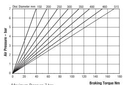
Maximum Pressure 7 bar Maximum Braking Force = 0.72kN@ 7 bar Weight of caliper and thruster - 0.8kg Weight of thruster only - 0.05kg Volume displacement of thruster at 6mm stroke = 4ml
