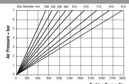
Maximum Pressure 7 bar Maximum Braking Force = 6.9kN @ 7 bar Weight of caliper and thruster - 8.32kg
