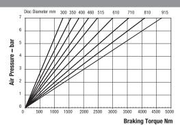
Maximum Pressure 7 bar Maximum Braking Force = 11kN @ 7 bar Weight of caliper and thruster - 9.06kg
