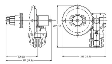
Maximum Braking Force = 6kN Weight of caliper and actuator - 15.7kg
