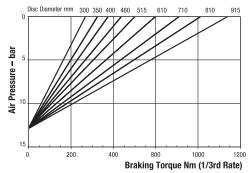
Minimum Pressure for full retraction: 17 bar Maximum Braking Force 1/3rd rate: 2.2kN Weight of caliper and thruster - 11kg
