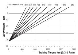
Minimum Pressure for full retraction: 33 bar Maximum Braking Force 2/3 rate: 4.3kN Weight of caliper and thruster - 11kg
