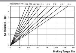
Maximum Pressure 7 bar Maximum Braking Force = 0.74kN @ 7 bar Weight of caliper and thruster - 7.34kg
