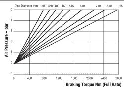
Minimum Pressure for full retraction: 5 bar Maximum Braking Force full rate: 6.4kN Weight of caliper and thruster - 10.5kg
