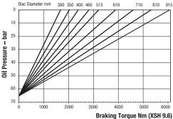
Minimum Pressure for full retraction: 82 bar Maximum Braking Force XSH 9.6: 14.3kN Weight of caliper and thruster - 11.6kg Weight of thruster only - 4.6kg Volume displacement of thruster at 6mm retraction = 9.1ml
