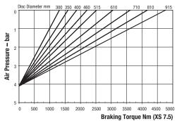
Minimum Pressure for full retraction: 5.5 bar Maximum Braking Force XS 7.5: 11.2kN Weight of caliper and thruster - 11.9kg Weight of thruster only - 4.9kg Volume displacement of thruster at full retraction = 1.19 l
