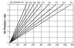
Maximum Pressure 7 bar Maximum Braking Force = 3.6kN @ 7 bar Weight of caliper and thruster - 8.15kg
