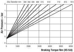
Minimum Pressure for full retraction: 6.4 bar Maximum Braking Force XS 9.6: 14.3kN Weight of caliper and thruster - 12.1kg
