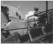
Wichita 15-1/2" mechanical PTO provides long service life for Cummins 855 diesel on rock crusher.
