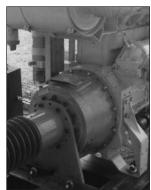
Wichita PTO mounted on Caterpillar diesel engine.
