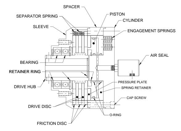
PARTS DIAGRAM FOR MODELS: E5D3K-STH, E6D3K-STH, E8D3K-STH, EAD4K-STH, EBD4K-STH
