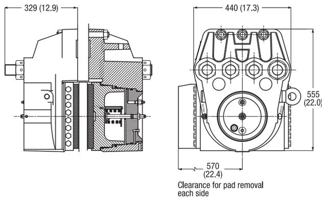
The Twiflex VMH2 disc brake caliper is comprised of two modules bolted to a central mounting plate, 12mm thicker than the brake disc. Minimum disc thickness is 38mm and minimum disc diameter is 1500mm with no maximum except for practical limitations.
