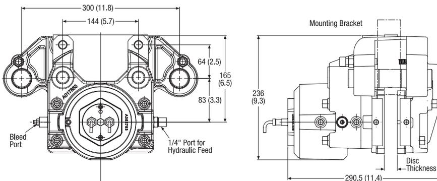
The Twiflex VKCS-FL disc brake caliper comprises a single spring module forming the 'active' side of this floating unit and is available for use where space is limited or to accommodate axial disc float of  $\pm 6$ mm.
