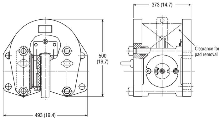
The Twiflex VH disc brake caliper is comprised of two modules secured between U-shaped top and bottom mounting plates by tie rods.
