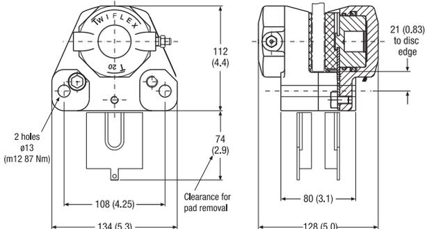
The standard Twiflex T20 disc brake caliper is split caliper design suitable for use with a minimum disc thickness of 12.7mm. Optionally, the caliper may be supplied in a modified form for use with a minimum disc thickness of 8mm. Normally the brake is side mounted, however, for use with a disc thickness greater than 20mm, the split design allows the modules to be mounted each side of a central mounting plate of the same thickness as the brake disc. Minimum disc diameter is 300mm.
