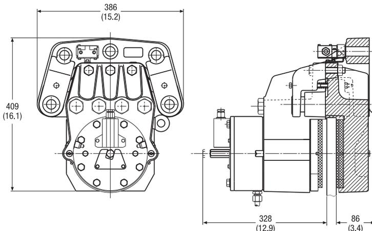
The Twiflex VKSD-FL disc brake caliper comprises a single spring module forming the 'active' side of this floating unit and is available for use where space is limited or to accommodate axial disc float of  $\pm 6$ mm.
