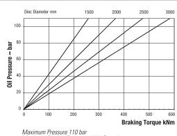
Maximum Presaking Force = 433kN @ 110 bar Weight of caliper ( 2 modules ) - 580kg Volume displacement per 1mm stroke at both pads = 101.5ml
