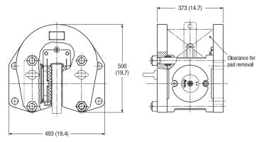
The Twiflex VH disc brake caliper is comprised of two modules secured between U-shaped top and bottom mounting plates by tie rods.
