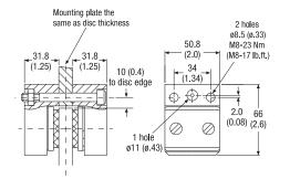
The Twiflex T2 disc brake caliper is split caliper design suitable for use with a minimum disc thickness of 5mm. The modules are mounted each side of a central mounting plate of the same thickness as the brake disc. Minimum disc diameter is 120mm. Alternatively, the brake may be side-mounted with a spacer equal to the disc thickness between the two halves.
