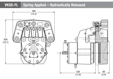
The Twiflex VKSD-FL disc brake caliper comprises a single spring module forming the 'active' side of this floating unit and is available for use where space is limited or to accommodate axial disc float of ±6mm.
