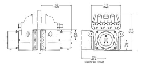
The Twiflex VMS3-SPS disc brake caliper is comprised of two modules bolted to a central mounting plate, 12mm thicker than the brake disc. Minimum disc thickness is 38mm and minimum disc diameter is 1500mm with no maximum except for practical limitations. Based on a development of the earlier Twiflex VMS2-SP disc brake, the VMS3-SPS provides a significant increase in braking force but in a similarly sized package.
