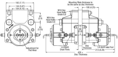
The Twiflex VCS Mk4 disc brake caliper is comprised of two halves, or spring modules, and is suitable for use with a minimum disc thickness of 20mm. The modules are mounted each side of a central mounting plate of the same thickness as the brake disc. Minimum disc diameter is 500mm.
