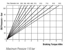
Maximum Braking Force = 20kN @ 110 bar Weight of caliper - 5.82kg Volume displacement per 1mm stroke at each pad = 4.8ml
