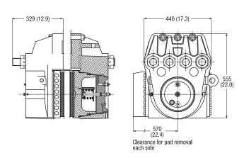
The Twiflex VMH2 disc brake caliper is comprised of two modules bolted to a central mounting plate, 12mm thicker than the brake disc. Minimum disc thickness is 38mm and minimum disc diameter is 1500mm with no maximum except for practical limitations.
